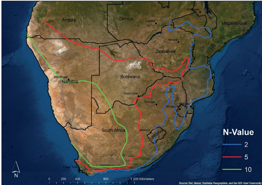
Fig. 11 Weinert N-values for southern Africa. Based on Jordaan, G.J., Kilian, A., Muthivelli, N., Dlamini, D., 2017. Practical application of Nano-technology in roads in southern Africa, in: Proceedings of the 8th Transportation Technology Transfer (T2) Conference, Lusaka, Zambia . pp. 8–10.
