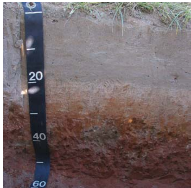
Figure 1. An example of the light-grey, silty, structureless topsoil overlying a thin mixed zone (20 centimetres to 30cm in depth), and then the more usual red clay derived from basalt.
